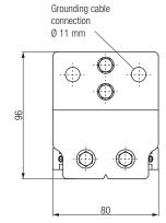
Part No.: 05-Z009-0004 • Grounding cable 16 mm<sup>2</sup> with
