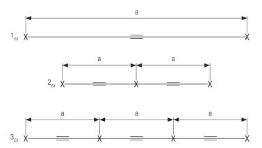
$a=\mbox{distance between anchor points} \rightarrow \mbox{arranged symmetrically as much as possible} \\ \mbox{Segments with E-RTG pickup guide deviate from this} - \mbox{see table for figure "a" on top} \\$
