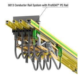
The illustration above shows that the dual function of the ProfiDAT® Profile results in a compact and fully integrated solution. Furthermore, it clearly shows that an existing ground conductor rail can be replaced by the ProfiDAT® System without additional space requirements or attachments.
