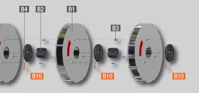
For the mentioned operations, you will need to remove 1 to 4 coupling disk **B4** (on the left: example for 4P type where 4 x **B4** are needed).
