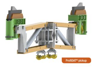
The ProfiDAT® antenna is an integral part of the current collector head. It moves inside the ProfiDAT® profile and is in contact with the mobile transceiver. Corresponding transceivers for each side have a standard Ethernet interface and are placed in the E-rooms or in separate control panels.
